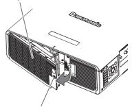
Lamp unit cover fixing screw
